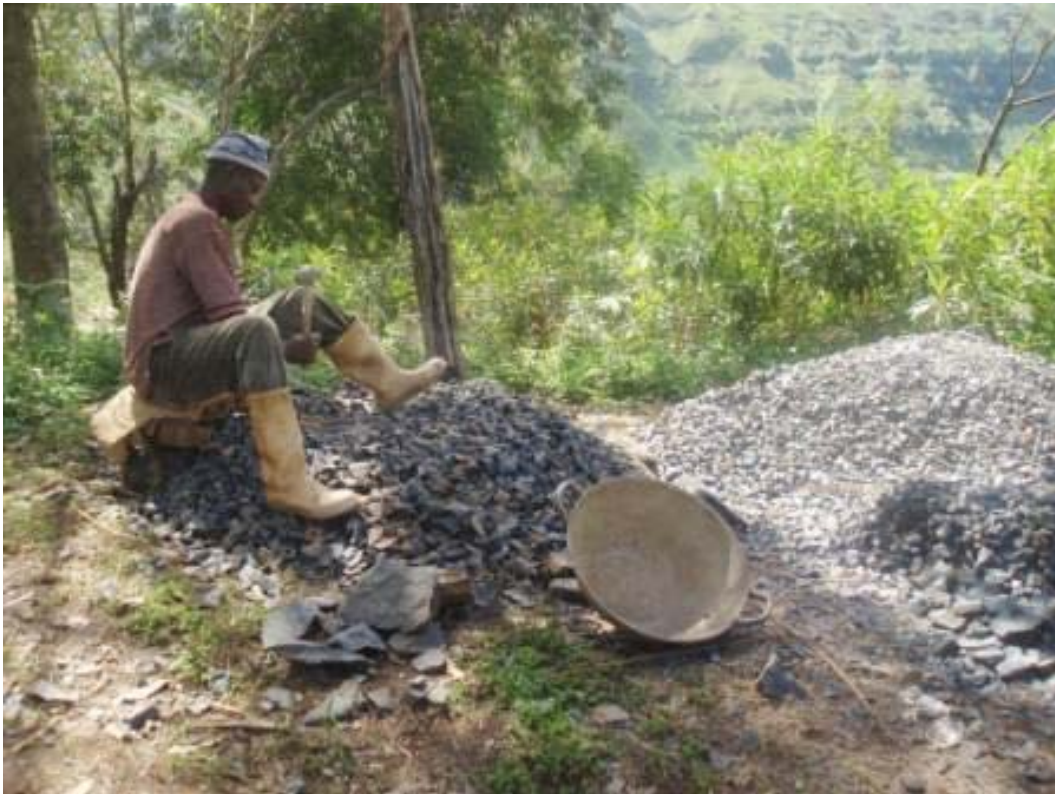
A worker shaping stones and crushing gravel/concrete (small pieces)
